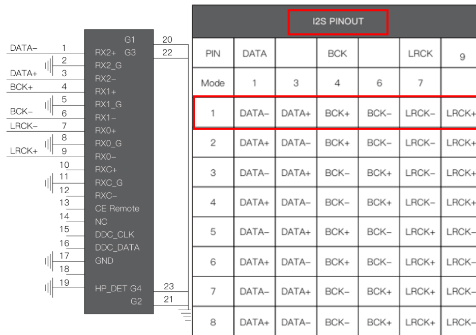
DENAFRIPS TERMINATOR解码器说明书给出的线序
